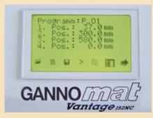
Electronic controller with touchscreen LCD-display. A program is choosen either by entering the program number or by barcode (optional).
