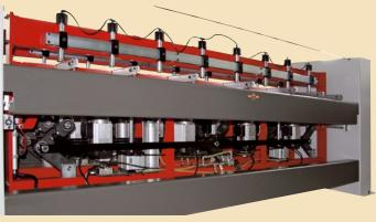
The drilling motion is completely controlled hydraulically for a constant feed speed and chip free boring on most coated panels. The through boring of the workpiece with no chip out reduces production time by approx. 65% for partitions.
